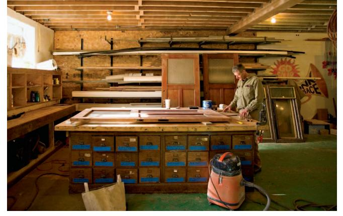
Charles Shaw in his basement workshop, sanding and refinishing salvaged doors for installation inside the Smiley Building. Much of the carpentry and other work for the restoration have been carried out here.
